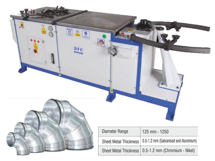
All cylinder are driven, high quality hydraulic component, Two can work in one machine at the same time with seaming and seam closing. 2379 cold set steel used which is resistant for high abrasion and high pressure. 50.000 hours abrasion — proofing except user error. The machine has installation, start-up, and on site service.
