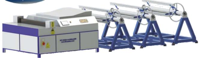
Square Duct Machine works 0.4 - 1.25 galvanised sheet metal and 0.4 - 0.8 chromium nickel thickness. The product dimension adjusted through operator panel and manufactured with high precision. You can manufacture square duct by help of powerful feeding motor and precise automation panel. 3 Roll carriers which is given with the machine helps the use needed roll. Line pattern, trapez pattern and a needed mark pattern is available.
